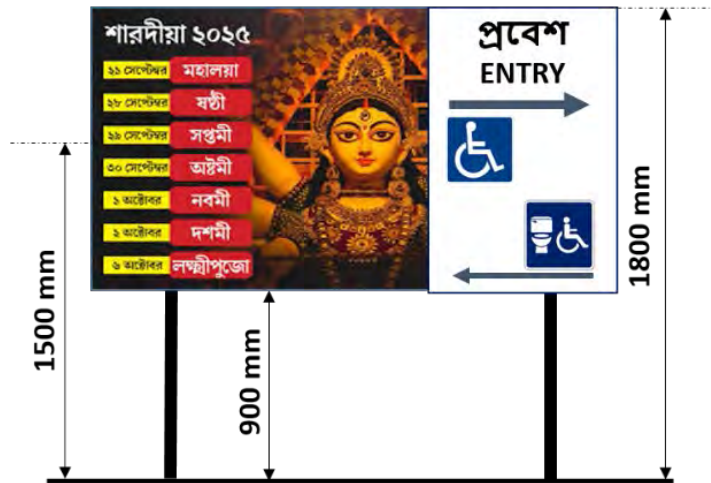
Fig. 2.17 Dimensions for placing an accessible sign-board
